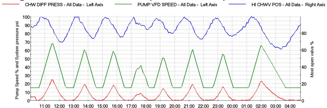
**Figure 2: Stable demand-based pressure reset loop**
