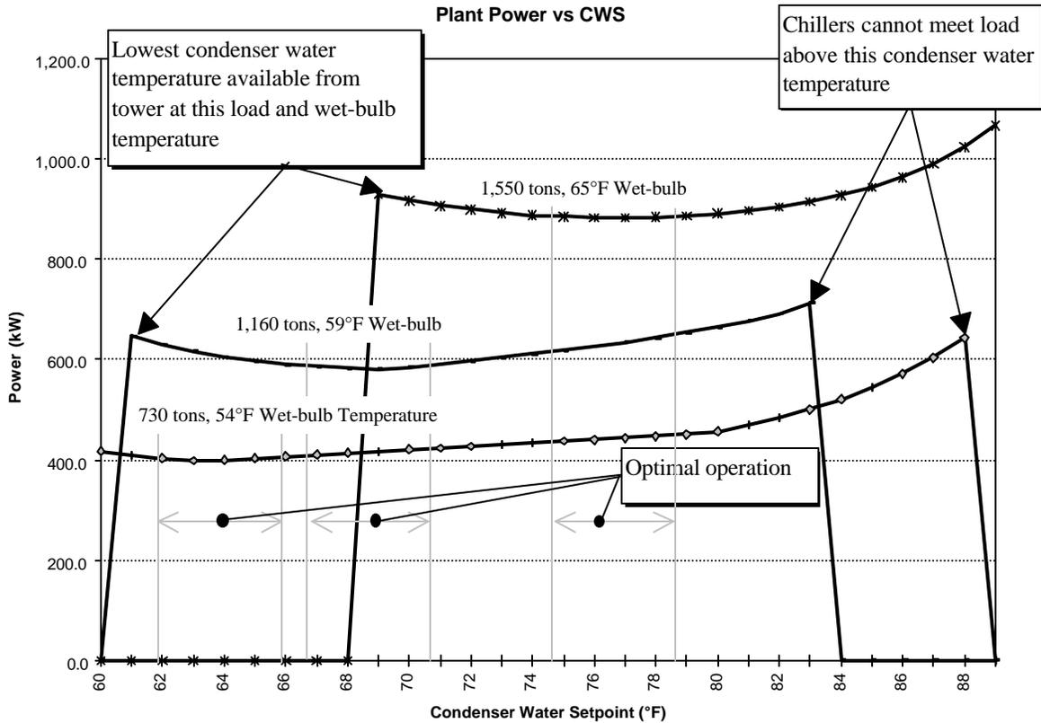
**Figure 5: Chilled Water Plant Power as a Function of Condenser Water Set Point.**
