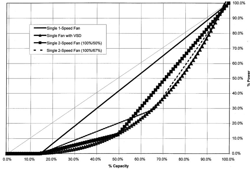
**Figure 1** The percentage power versus percentage heat rejection capacity of single-speed, two-speed 100%/50%, and two-speed 100%/67% fan controls.
