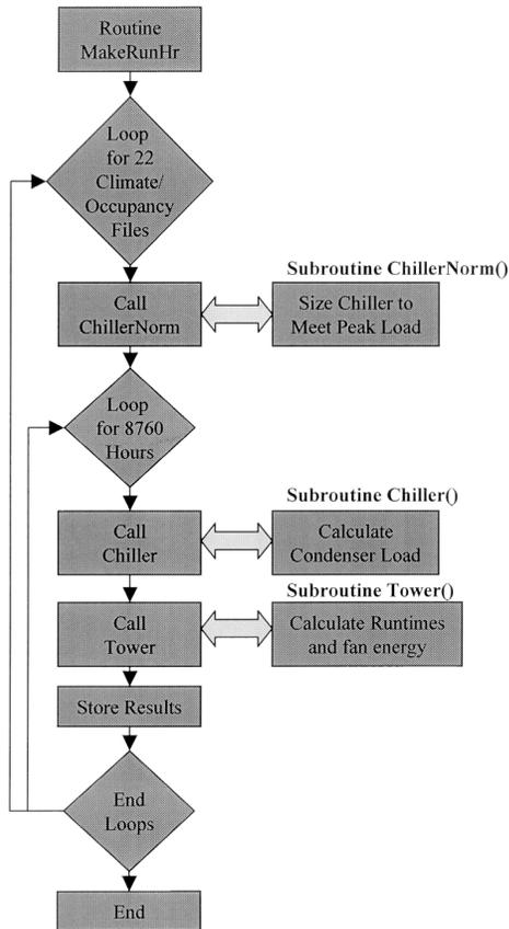
**Figure 2** The central plant computer model calculation flow diagram.
