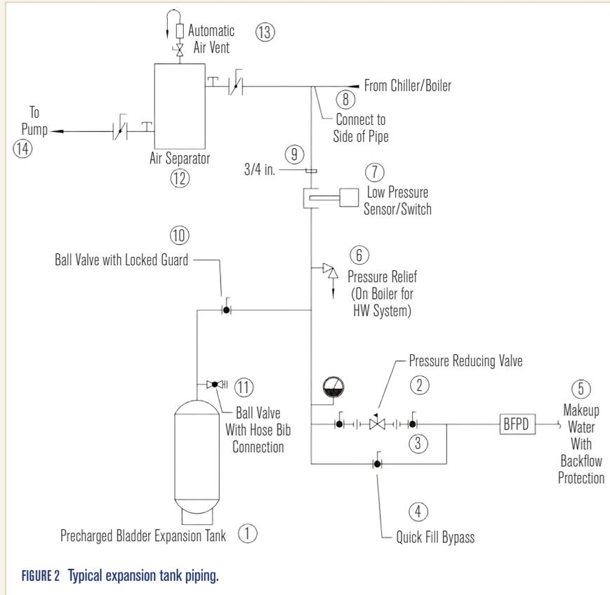
FIGURE 2 Typical expansion tank piping.
