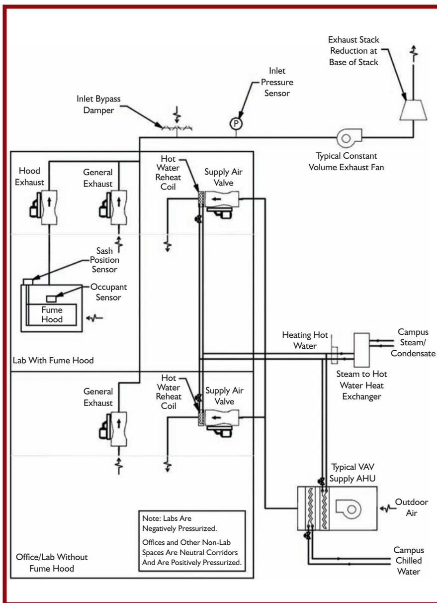
Figure 1: Stauffer I chemistry laboratory VAV retrofit system.
