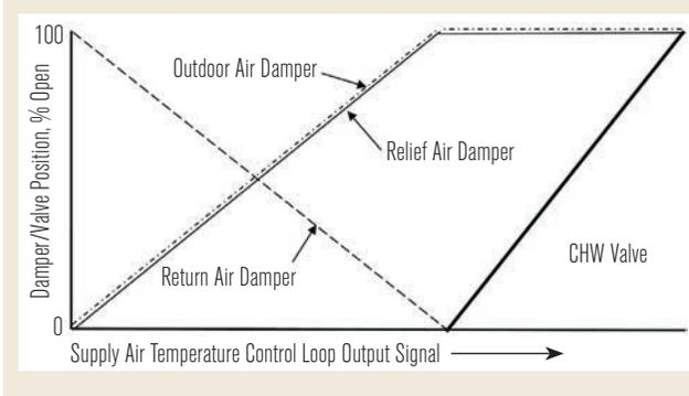
FIGURE 5 Economizer damper control for systems with relief dampers or relief fans.
