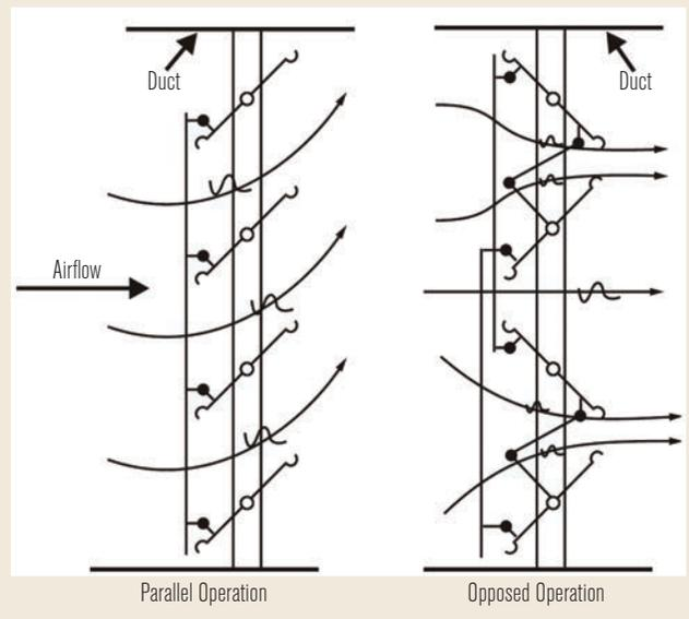
FIGURE 8 Mixing box pressure drop with opposed blade vs. parallel blade mixing dampers. (Adapted from References 9 and 10.)
