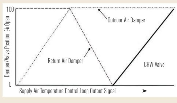
FIGURE 6 Economizer damper control for systems with return fans and airflow tracking control.
