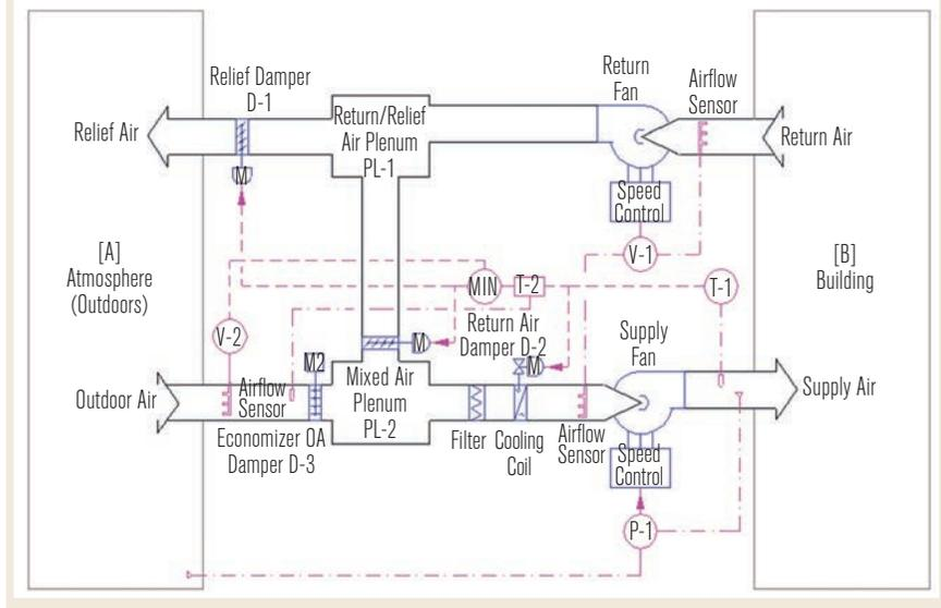
FIGURE 3B Return fan with direct pressure control.
