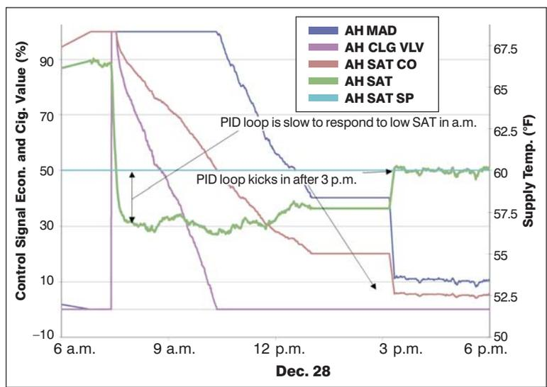
Figure 3: Trend review of air-handling unit cooling loop.
