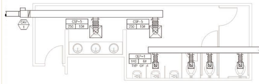
FIGURE 2 Better restroom exhaust and makeup system design.
