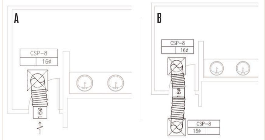
FIGURE 6 Transfer air plus cooling supply options.
