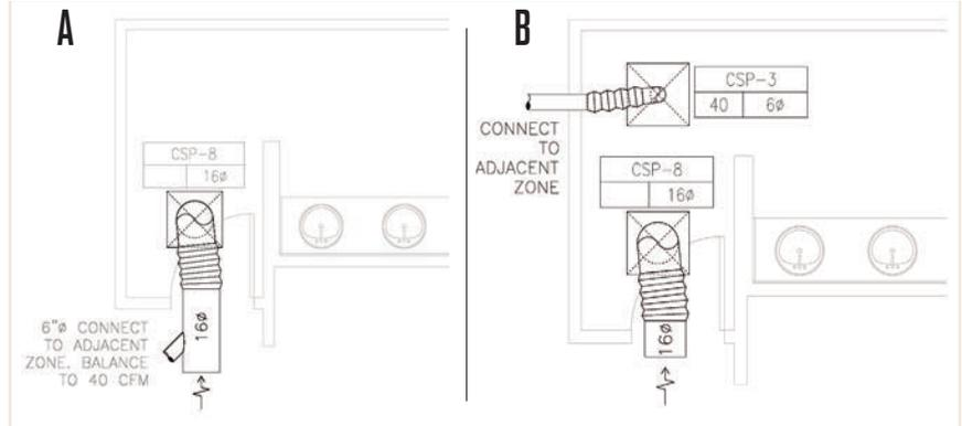
5. Ducted transfer to ceiling return air plenum with separate supply air (Figure 6b). If the design in Figure 6a is felt to be too confusing, conditioned air may be supplied by a separate diffuser. This option is more expensive than Option 4 but easier to understand and to balance.
