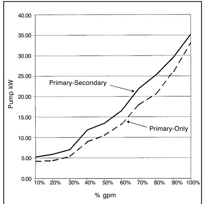
**Figure 3: Pump energy for primary-only and primary-secondary systems in three chiller plants.<sup>†</sup>**
