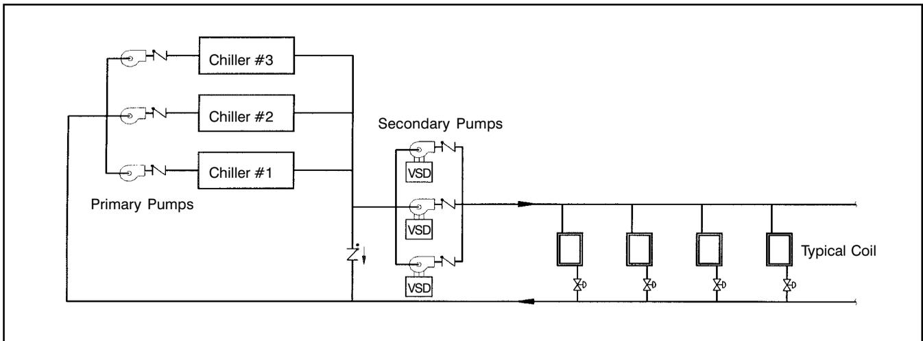
**Figure 2: Conventional primary-secondary system.**
