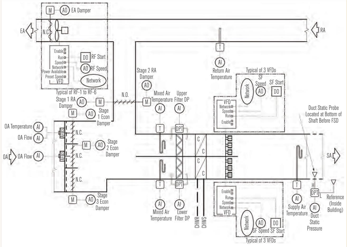
outdoor air damper control, two with OAFMS, and two stages of return air damper control.
