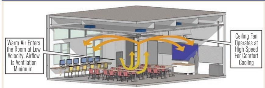
FIGURE 3 Heating with automatic ceiling fan assistance (cold weather).
