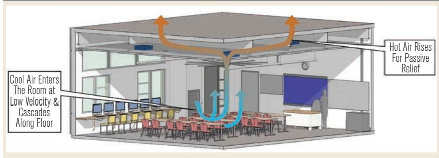
FIGURE 2 Cooling by automatic ceiling fan (warm weather).
