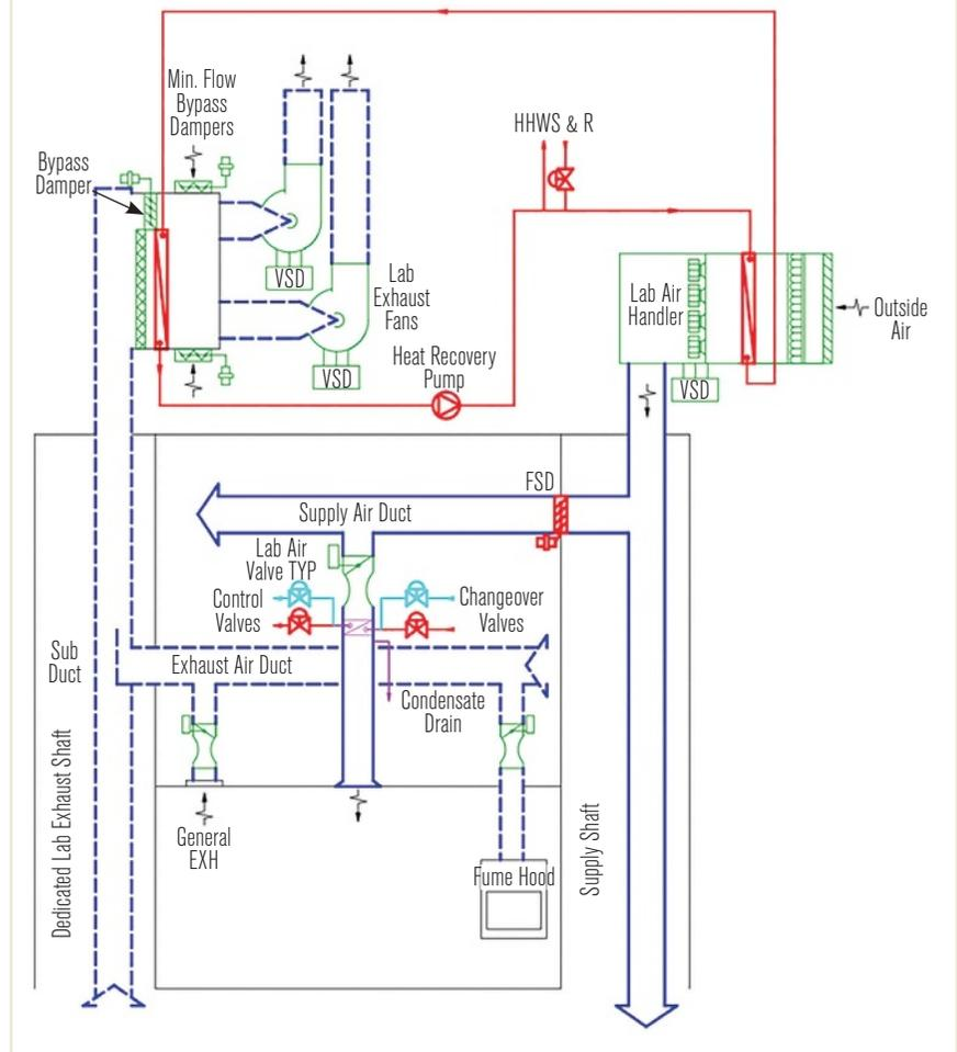
Sizing the outdoor air system for the loads in load-dominated labs also improves flexibility – hoods could be added to the lab in the future with nothing more than setpoint changes to the outdoor air supply system.
